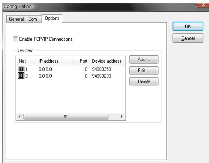
By activating the option 'Enable TCP/IP Connections', the driver will communicate via TCP/IP.
